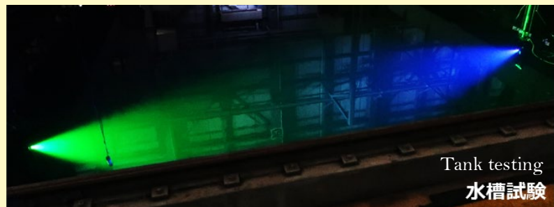
Tank testing of hybrid opto-acoustic underwater wireless communication Provided by: ATLA
