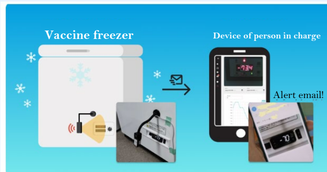
Figure 1-4-3/Freezer temperature control system that uses the IntegrAI Camera
