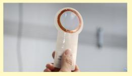
CO2 permeable membrane of 34 nanometer Provided by: Kyushu University
