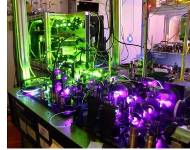
Optical lattice clock Source: AIST
