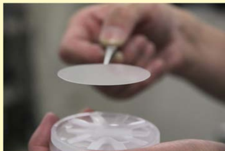
Wafer of GaN crystal with few defects (circular thin plate made of crystals of semiconductor material)
