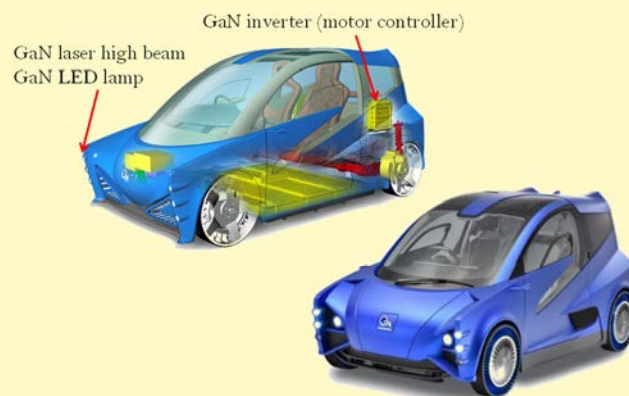
Outline figure of electric car using GaN (upper left) and a real machine exhibited at Tokyo Motor Show 2019 (lower right)
