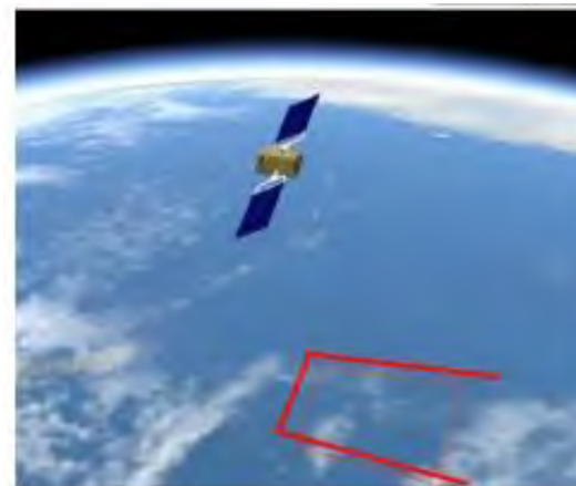
One camera large swath (120Km) and low resolution (30m at 500km orbit) in red
