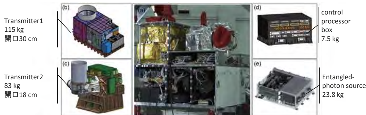
FIG. 18 The full view of the Micius satellite and main payloads. (a) The photograph of the Micius satellite before launching. (b) The transmitter 1 for QKD, entanglement distribution and teleportation. (c) The transmitter 2 specially for entanglement distribution. (d) The experimental control box. (e) The entangled-photon source.
