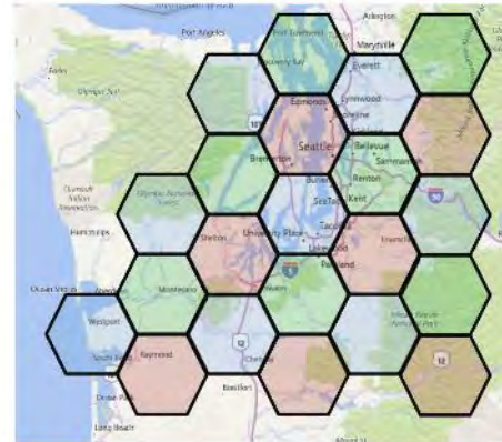
Representative Spot Beam Frequency Reuse (300km 2 Spot Area)
