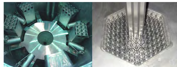
Figure 3: Assembled and installed NSC KIPT neutron source core with target.
