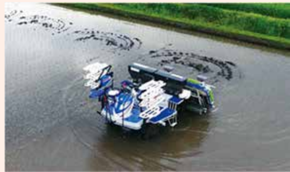
Automatic driving rice planting machine under unmanned operation
