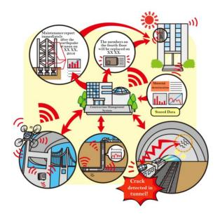
inspections and repairs. Based on the data collected by inspection robots regarding deterioration of, and damage to, these roads, tunnels and bridges, the system determines the appropriate timing and details of repairs by taking into account priorities among these facilities.
