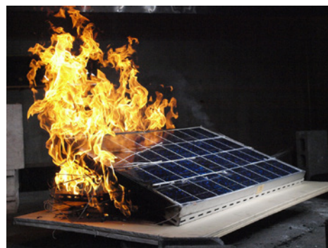
Fire exposure experiment of a solar cell module Source: NRIFD
