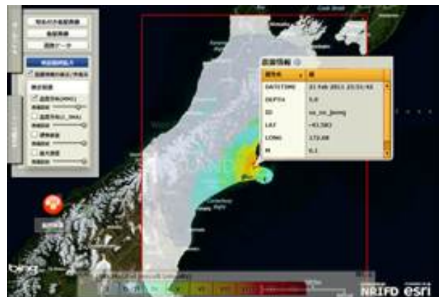
Example of display of earthquake damage estimation system (FDMA) Courtesy of National research Institute of Fire and Disaster
