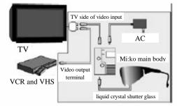
Image 1: 3D stereoscopic viewing system
