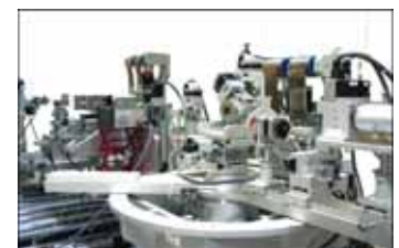
High precision parallel x-ray micro-beam formation equipment
