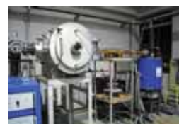
Sintering machine for ceramic materials using submillimeter wave
