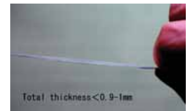
Sheet type all solid state lithium secondary battery prototype
