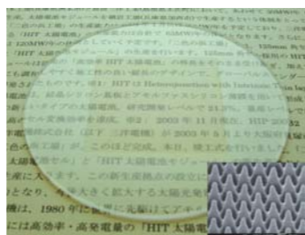
Anti-reflection structured surface (patterned part, 50 x 50 mm; SANYO Electric Co., Ltd.)
