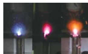
Light emitted from in-liquid plasma including metal salts
