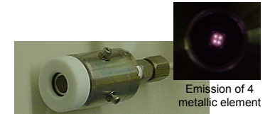
Opposed type multi-element monitor light source (diameter: 34 mm, length: 40 mm)
