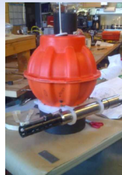
Deep SOLO SIO 0 – 6000 m SBE-61 CTD 25 kg 33 cm glass sphere 3 deployed
