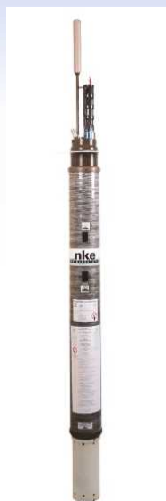
Deep ARVOR NKE社, CNRS & IFREMER 0 – 4000 m SBE-41 CTD 26 kg 8 deployed
